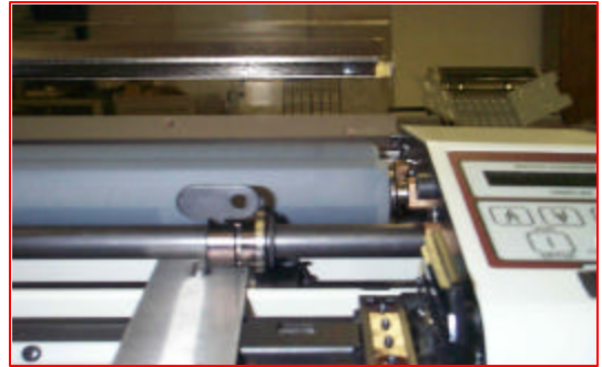
Compression tool Installed
