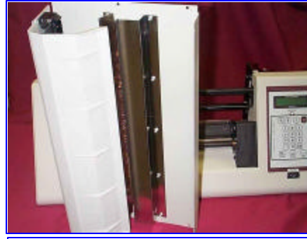
Bezel assembly is the hood, back and bottom of the machine in one
