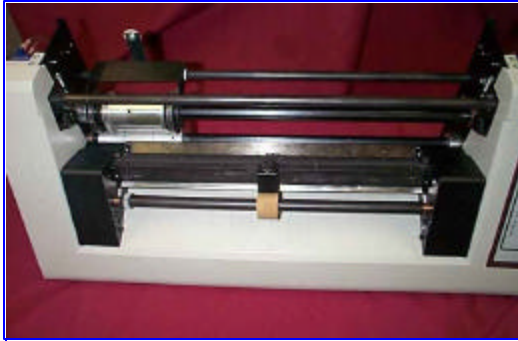
Remove both side covers and bezel assembly before removing feed drive.
