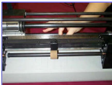
Disconnect the paper sensor from behind, before attempting to remove the feed assembly.
