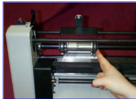
Components must be moved to the side to access the paper sensor.
